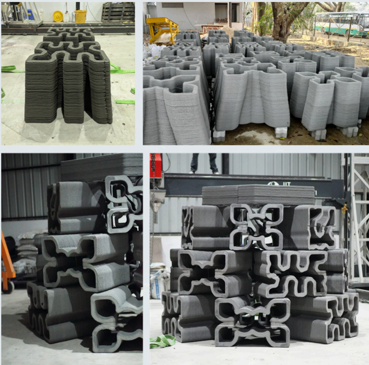
Fig. 1 Fabrication of 3D-printed artificial reef modules at IIT Guwahati
